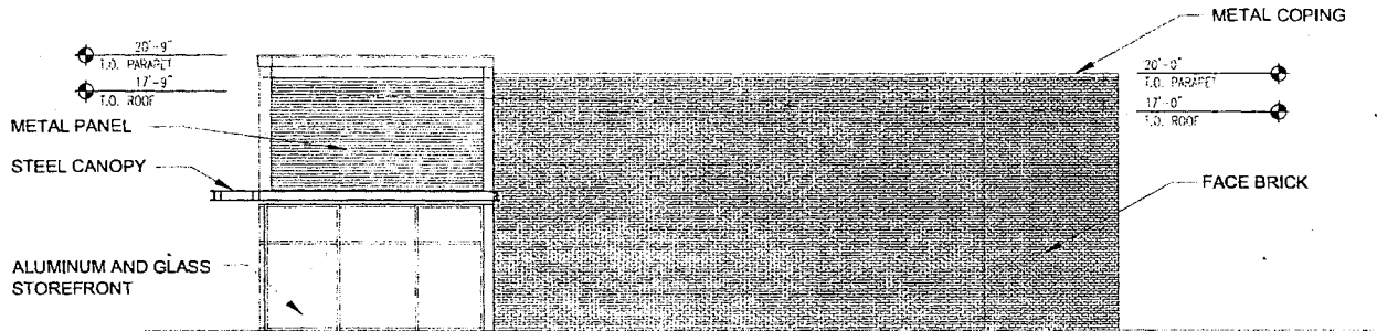
RETAIL A7 - SOUTH ELEVATION SCALE: 1/8" = 1'-0"
